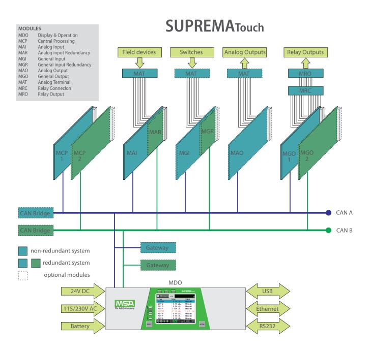
Only seven basic modules are necessary to provide full functionality, namely MCP20, MDO20, MAI30, MGO20, MGI30, MAO20 and gateways.
